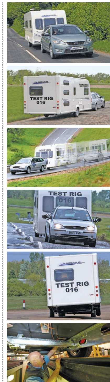
Pictured from top: Pegasus on the road; all the prototypes were subjected to being towed over a section of Belgian pavé – replicating some of the worst roads in Europe; the speed test at the Millbrook Proving Ground; speed humps like you've never seen before; the potholes at Millbrook are far more severe than anything a caravan is likely to meet on normal roads; at regular intervals during testing, the caravans were given a thorough inspection by Millbrook staff
