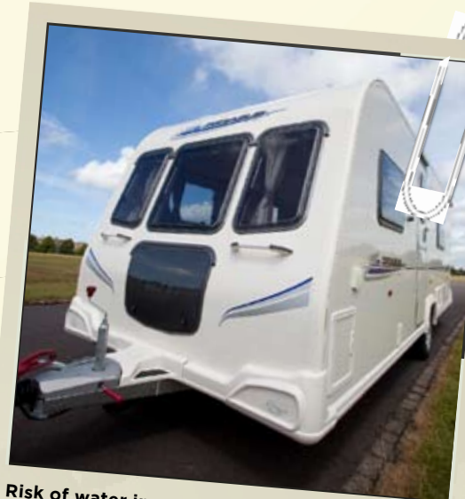
Risk of water ingress is minimised by the single panel forming the roof and front of the van, eliminating the need for a joining seam
